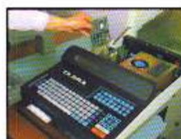
The TMM Comes Complete With an Alphabet/Function Keyboard Including Built-In Dual Disk Drives and a Paper Tape Reader
